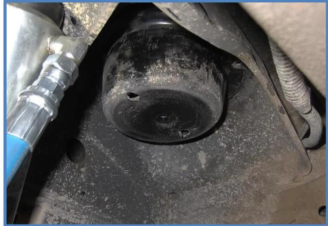
3. Using a 2 1/4" hole saw, cut a hole in the center of the bump stop mount using the threaded hole in the center as a guide for the pilot bit.
