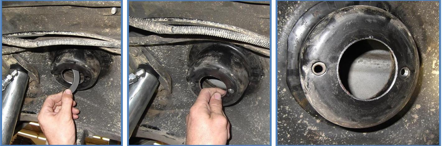
5. Install bump stop brackets – Line up holes in brackets with the nut plate and install the 3/8 x 1” bolts with washer, be sure to use red lock tight. Tighten bolts to 35 ft/lbs.
